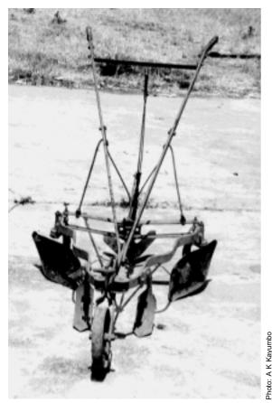
Figure 4: Cultivator fitted with reversible front tines, hiller blades and rear sweep
