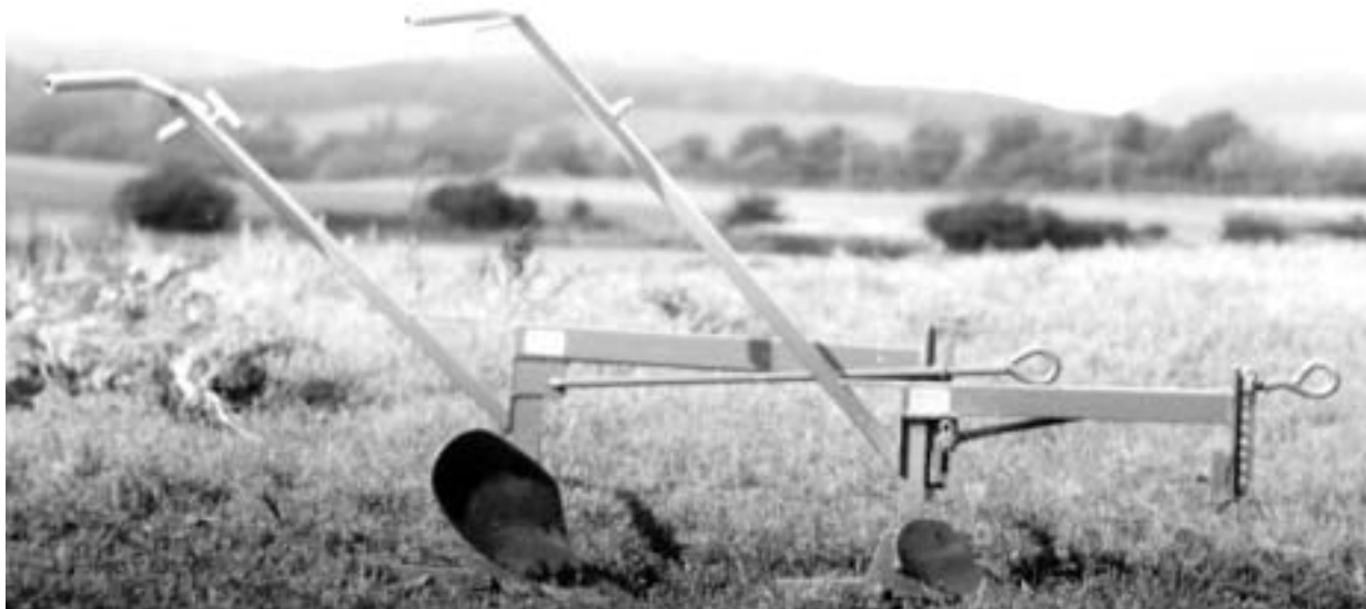
Figure 2: 6" EC1 plow (left) and earlier model of the 4.5" single donkey plow
