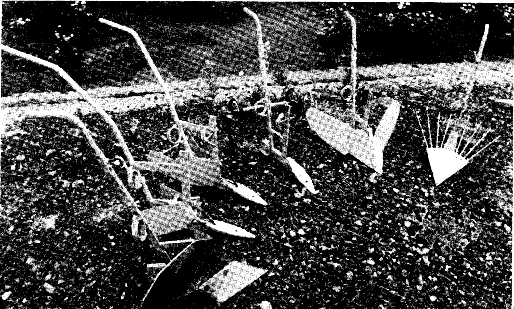
Photo 2: Prototype implements made at Selam workshop. Based on Latin American designs, they fit onto a long wooden beam. From bottom left to right: mouldboard plow, chisel plow, ridger, cultivator, ridger and potato lifter
