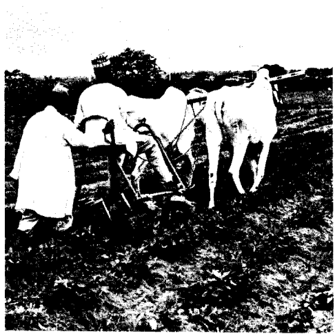
Fig. 2: On-station testing of IAR straddle-row weeder.
